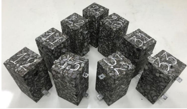
Figure 3.1. Preparation of samples for AC, PMB, HiMA mixtures.
